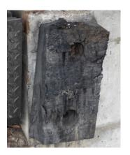
With up to 80,000-lb. trucks backing (and banging) into loading docks, the need for protection against repeated impact inspired the adoption of the dock bumper. In the 1950s, bumpers were fashioned from blocks of hardwood or molded rubber. However, as dock traffic increased, these materials proved to be inadequate as they required far too frequent replacement.
